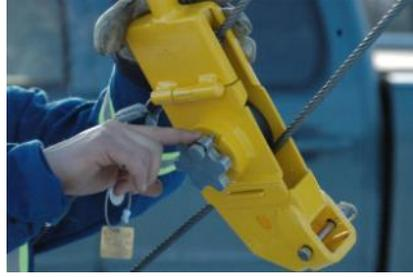
2.10.4. Close the sheave gate & tighten the sheave gate knob clockwise until snug. Turn the lock-pin knob until it drops into the lock position (DO NOT use wrenches to tighten). Inspect the sheave gate's locator flap for damage & for proper fit.
