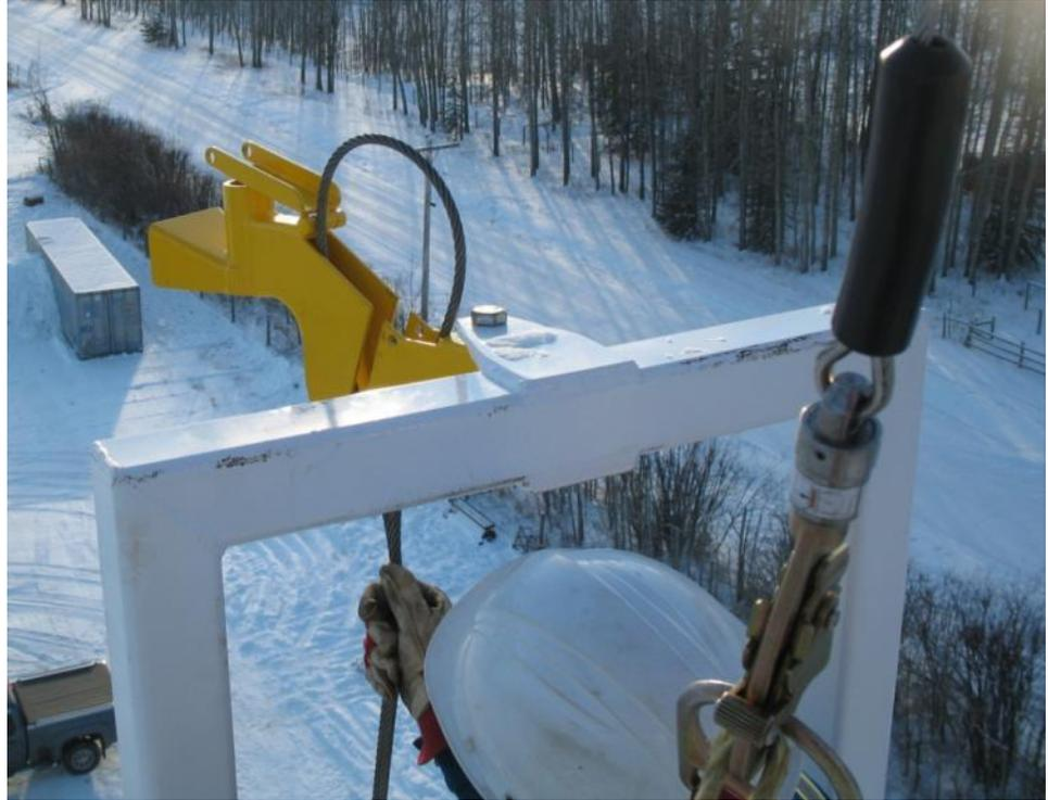
2.3.2.11. Create a 180° return bend on cable and push it through the underside of the Snubscape docking station until the 180° returning bend is exposed about 6” through the sheave gate opening.
