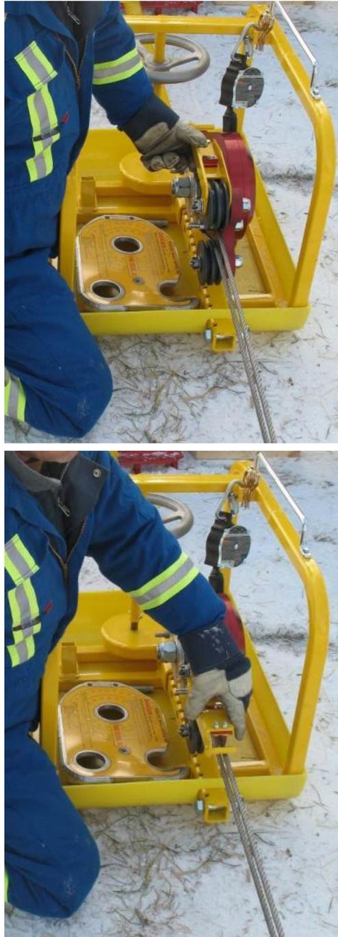
2.8.1. Rotate out the tension indicator. Side slip the cable across the back stop pin until the cable slips to the top of the back stop pin.
