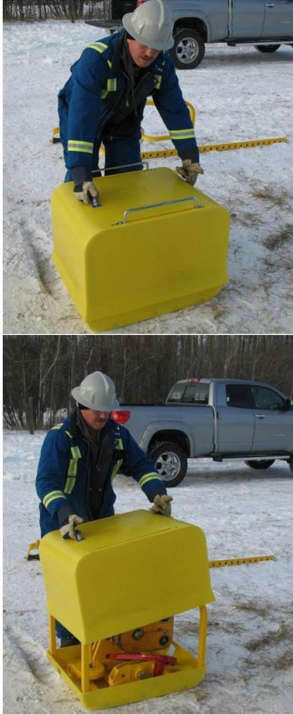
2.4.4. Remove the protective cover, exposing the Magnegress system.
