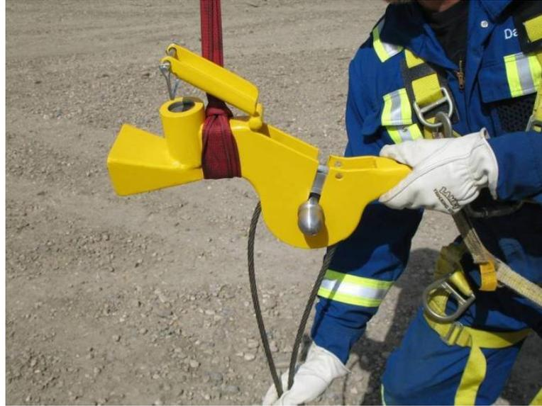
2.3.1.10. Draw or pull both the cable & sheave until the sheave pin is completely bottomed out in the slot.
