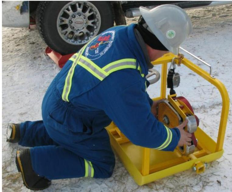
2.7.1. Remove the sheave cover plate from Magnegress brake housing.
