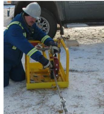
2.7.8. Cable must line up with corresponding idler sheave grooves when installed on the drive sheave.
