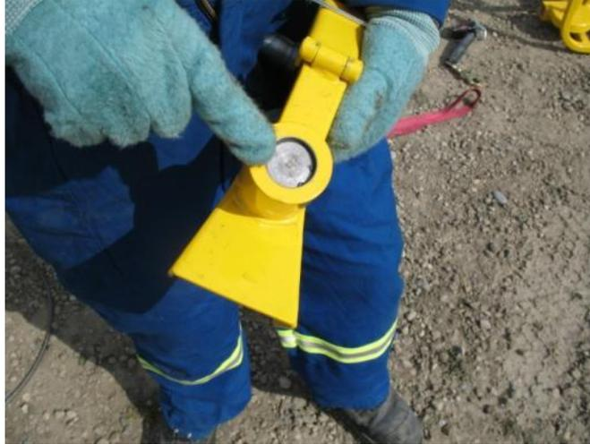
2.3.1.1. Ensure the spring clip is installed correctly & undamaged in the docking station magnetic pocket.
