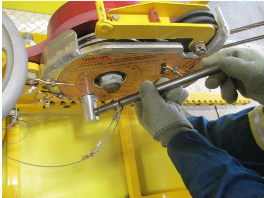
2.9.7. Insert handle into the override-brake hub.
