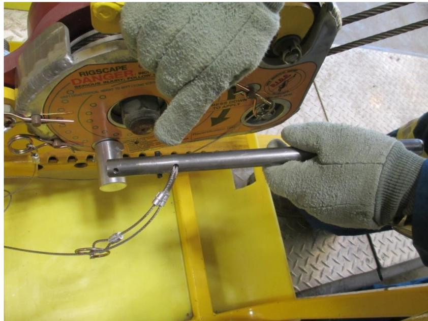
2.9.6. Check to see that the spring pin is properly inserted into the override-brake handle.
