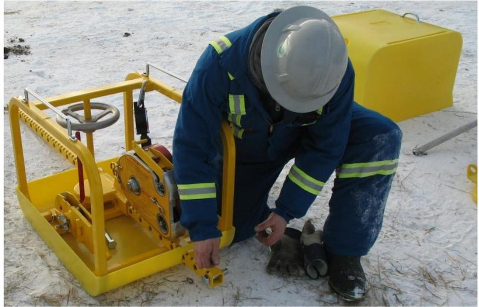
2.4.7. Insert the stopper bolt, nut & safety pin.
