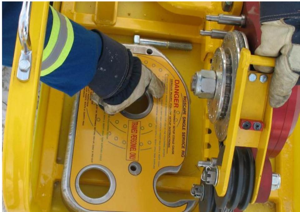
2.7.4. Install the cable on the proper sized sheave as per cover plate decal.
