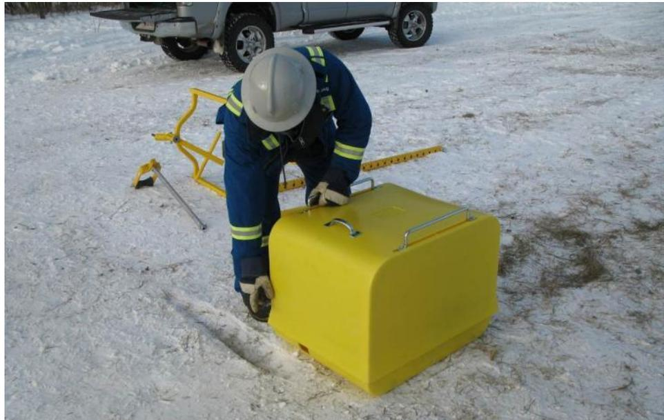
2.4.3. Position the back of the Magnegress frame approximately in line to your mark on the ground.
