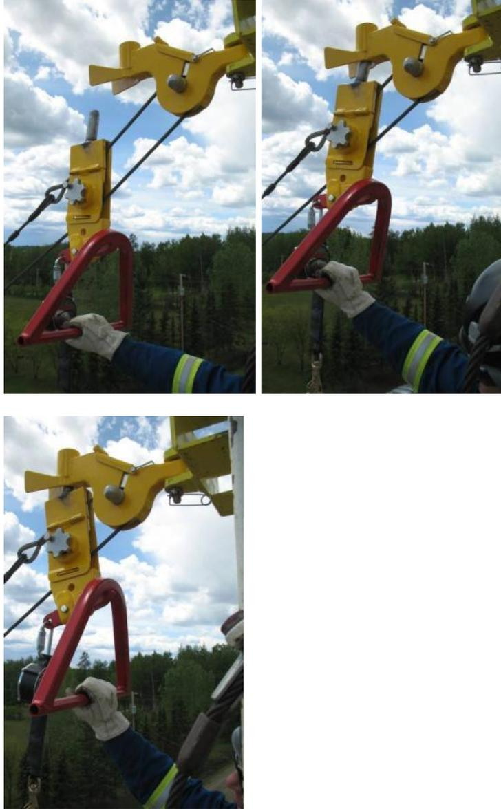
2.11.2.2. Guide the docking pin on the trolley housing into the docking station's receiver tube.
