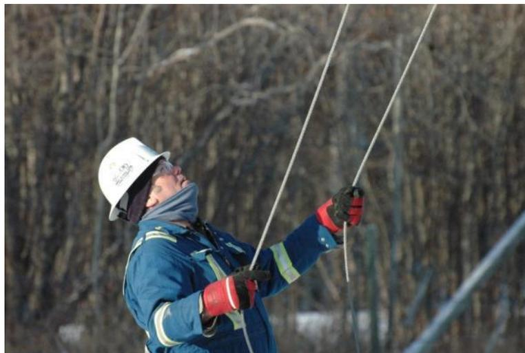
2.7.2. Standing directly in line with the Snubscope docking station, ensure the cable is not twisted, by holding each part of the looped cable in each hand & extending your arms out to your sides spreading the looped cable apart.
