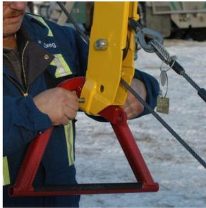
2.11.1. Insert the tri-handle into the trolley receiver tube & install the keeper bolt, nut & safety pin.
