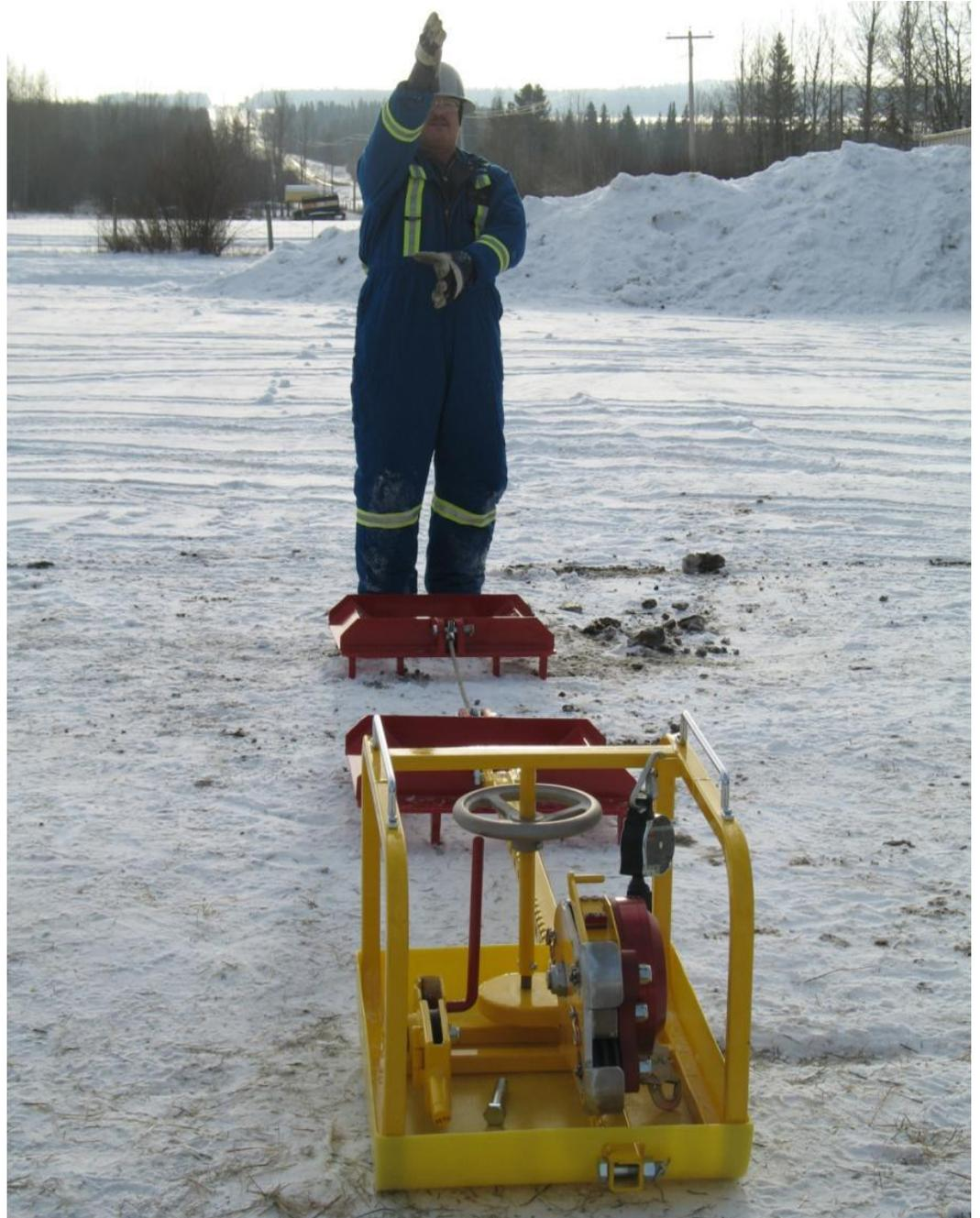
2.5.4. Align the Magnegress system to the top anchor point.
