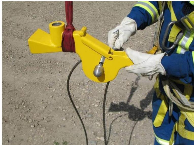
2.3.1.11. Flip down the sheave gate into its closed position & install the safety pin.
