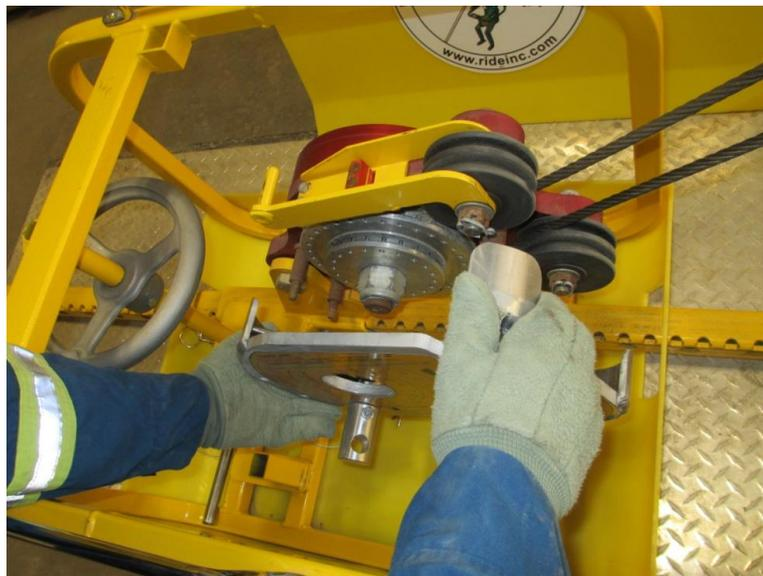
2.9.3. Place the cover onto the Magnegress brake system.
