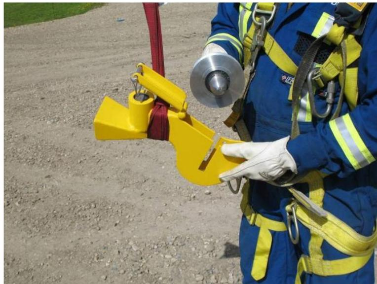
2.3.1.5. Open sheave gate & slide out sheave assembly.
