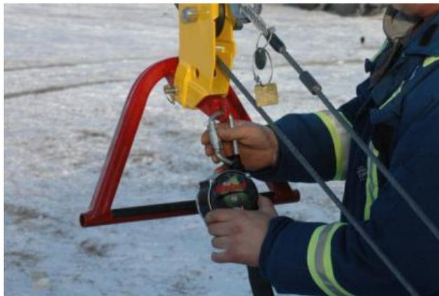
2.11.2. Attach the SRL (Self-Retracting Lanyard) into the SRL anchor point at the end of the tri-handle shank.
