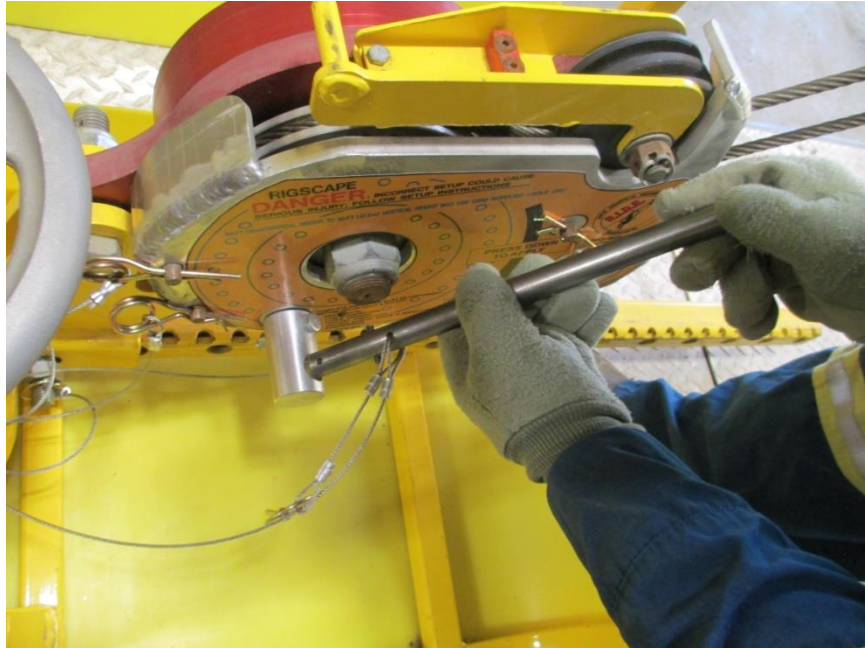
2.9.7 Insert handle into the override-brake hub.
