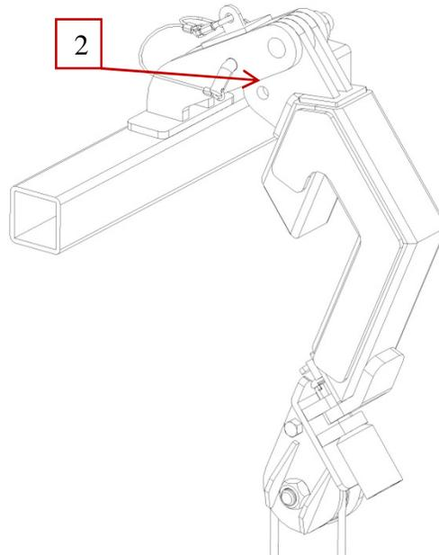
To place in transport mode, Remove the pins, lower the davit arm & re-install the pin (2) & keeper pin to prevent the pins & cables from getting entangled.
