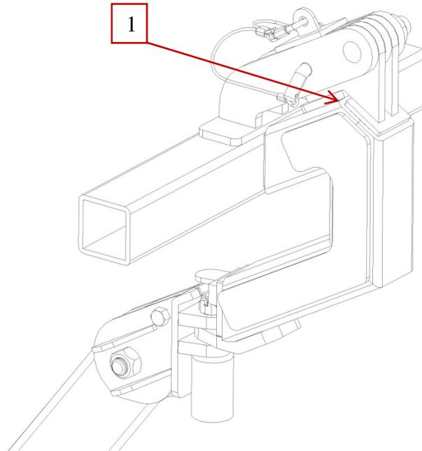
To place in working position, lift swinging davit into the work position & install main pin (1) & keeper pin. The Davit is now ready for use.
